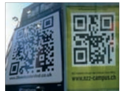
ILLUSTRATION 24: Billboards showing semacodes, or a form of 2D barcode matrix. Such codes, which are readable by most phone cameras, are a form of hyperlink in the physical world
